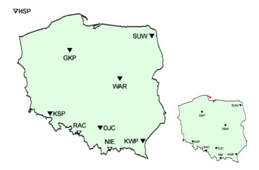
Broadband stations are black triangles, short period stations are open triangles. HSP is located well outside the map on Svalbard, here it is marked only schematically, i.e. that it exists.
