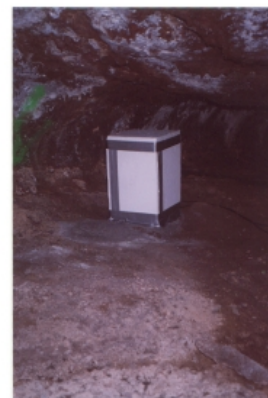
CMG-40T sensor with thermal insulation, inside the lava tunnel.
